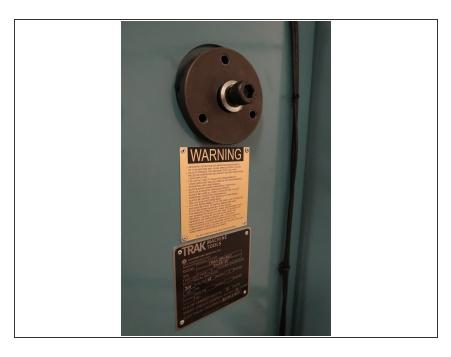
Once both the counterweight and column holes are center aligned, place the retaining plug that supports the counterweight into the column hole.
