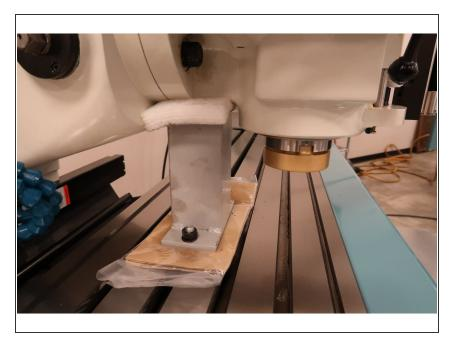
Jog the head down slowly on the Z-Axis until it bears down on the protective Styrofoam on top of the head shipping block.
