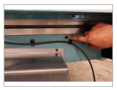
Once the head is tightly secured onto the head shipping block, use a 6 MM Socket to lock down the X Axis gibs tightly.
