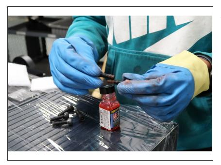
Apply threadlocker (<u>Loctite Blue 242</u> or equivalent) on the counterweight support screws to help keep them in place inside the column. Doing so will prevent possible vibration damage to the screws during transit.
