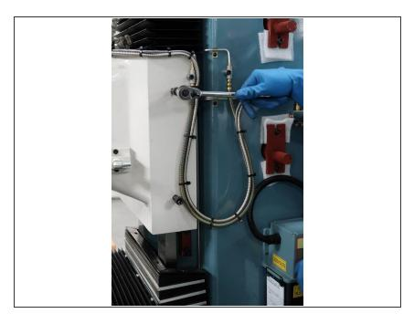
Moving on to the gibs section on the Z-Axis, use a 10 MM Hex Socket to center screw the two gib screws tightly.
