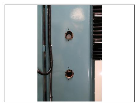
Align and center both counterweight holes to the column holes. You should be able to insert the two counterweight support rods through these holes without any obstructions.
