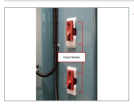
Place foam sheets behind each counterweight bracket against the column to prevent the bracket itself from scratching the column's paint.
