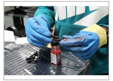
Apply threadlocker (<u>Loctite Blue 242</u> or equivalent) on the counterweight support screws to help keep them in place inside the column. Doing so will prevent possible vibration damage to the screws during transit.
