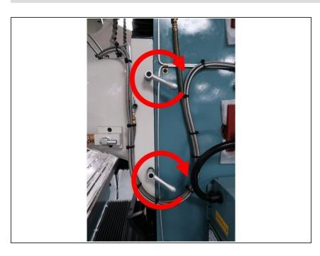
Once both holes are center aligned, lock the two ram gib locks tightly (located on the Z-Axis) by turning
